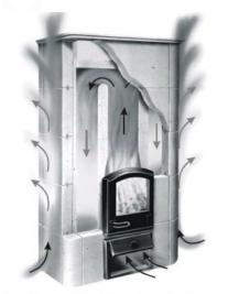
Operating principle of a masonry heater
